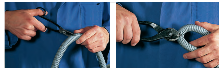
Kunststoff-Ummantlung durchschneiden Cut through the plastic sheathing
