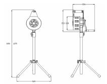
Maximum dimensions Stand height: max 1m, min 0.6m When folded: height 0.2m, base tripod 0.03m x 0.03m x 0.03m
