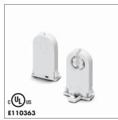
G13 push-through lampholders for lamps T8, T12 Pin support for reliable contact Lamp axis: 17 mm (0.67") Weight: 5,4 g, unit: 1000 pcs. Type: 26300/26302 with stop Ref. No.: 551271 Ref. No.: 551275 internally shunted Type: 26310/26312 without stop Ref. No.: 551272 Ref. No.: 551277 internally shunted
